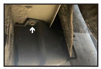
3. Using a 10MM socket, remove the one (1) bolt next to the wheel well on the driver side of the vehicle. Remove plastic piece and set aside to be reinstalled later.
