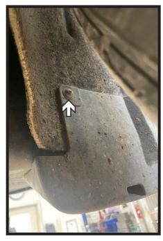
2. Using a Phillips screw driver, remove the one (1) screw from the rear wheel well on the driver side of the vehicle.
