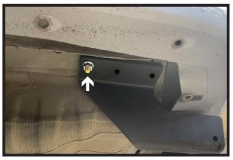
Feed lead wires through rear hole in receiver hitch on both sides. Raise hitch into place. Remove lead wires and loosely install 7/16" whiz flange nut onto each bolt. Leave loose.
