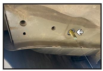
6. Attach lead wire to 7/16" carriage bolt and feed through hole in spacer plate. Insert bolt, then long end of spacer plate through hole in the frame. Ensure spacer plate is sitting flush against inner frame and the bolt is hanging vertically. Do this on both sides of the vehicle.
