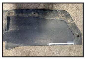
Using a reciprocating saw trim the plastic piece from the driver side of the vehicle as shown.
